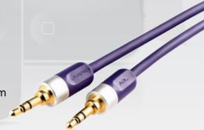
The iD-35 Series cables feature silver-plated  $\alpha$  (Alpha) OCC conductor for minimal transmission loss and 24k gold-plated connectors. The cable achieves superior noise isolation with two-layer shielding – aluminum foil and tinned copper -- in a RoHS-compliant sheath. The main conductors are treated with Furutech's  $\alpha$  (Alpha) Process – a deep cryogenic and demagnetizing treatment.
