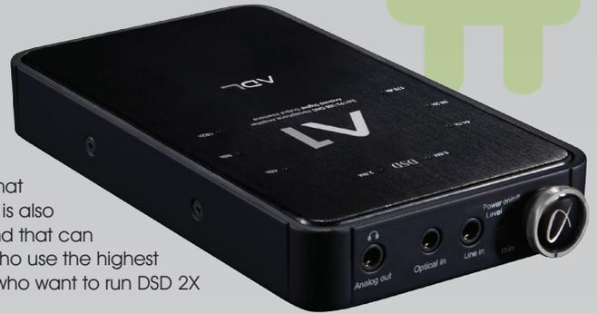
The new ADL A1 is a high-resolution portable headphone amplifier and DAC that can be used with Android devices such as ADL's own X1 and iDevices. The A1 is also DSD-capable when used with either Mac or Windows. The high-resolution sound that can be achieved through the A1 makes it perfect for portable audio enthusiasts who use the highest quality headphones to delve deeply into a recording. It's also ideal for those who want to run DSD 2X on either a laptop or a desktop.
